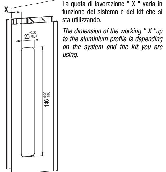
The dimension of the working "X" up to the aluminium profile is depending on the system and the kit you are using.
